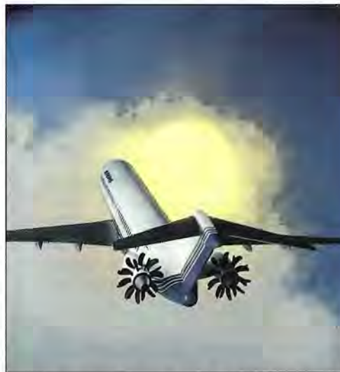
Though never put into production, the 7J7, with its distinctive ultra-bypass-engines, pioneered many technologies that found their way into the 777. Alan Mulally served as engineering director on the project, which sought to develop a highly fuel-efficient plane for 150 passengers.
